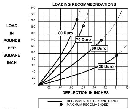
**SAMPLE** – 1/2" X 4" X 4" PIECE COMPRESSED BETWEEN NON-ADHERED METAL SURFACES.
